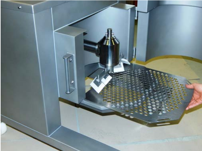
Fig. 27: Scraper unit placed transversely to the plate
