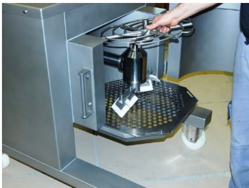
Fig. 15: Mounting the spiral separator Spiral separator mounted
