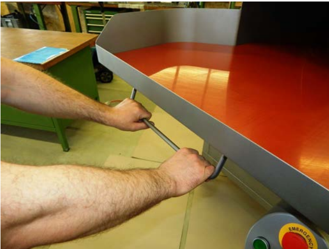
Fig. 24: Lifting the chute
