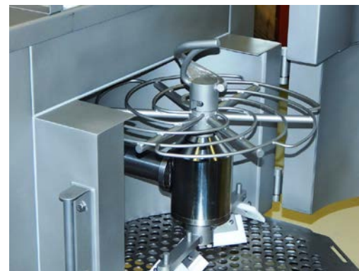
Fig. 18: Pre-separator hook mounted
