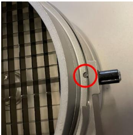
Fig. 32: Inserted dicer grid
