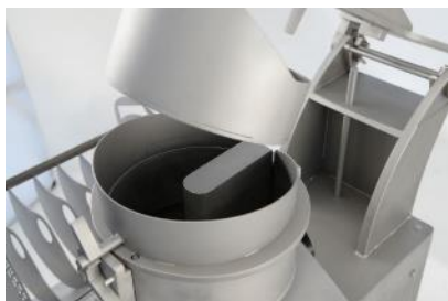
Fig. 38: Insert the neutral blade plunger
