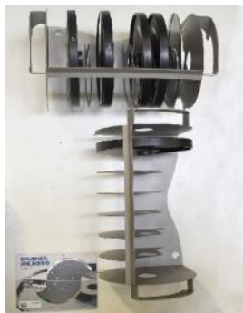
Fig. 41: Wall-mounted cutting disc holder
