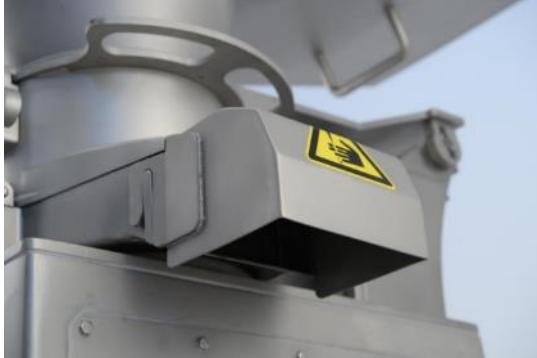
Fig. 35: Cover mounted onto the outlet
