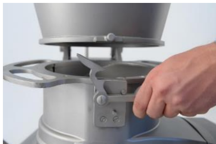
Fig. 23: Lock the funnel
