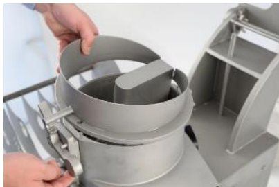
Fig. 37: Ring for the neutral blade
