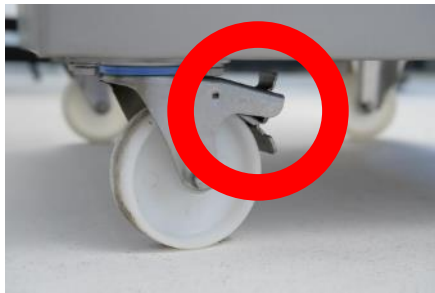
Abb. 14 Parking brake locked in place
