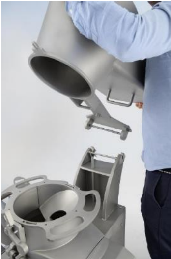
Fig. 19: Mounting the funnel
