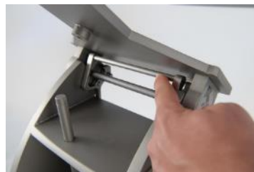
Fig. 22: Safety lock closed
