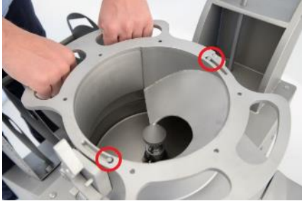
Fig. 18 Inserting the screw blade
