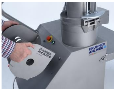
Fig. 42: Mounting the cutting disc holder
