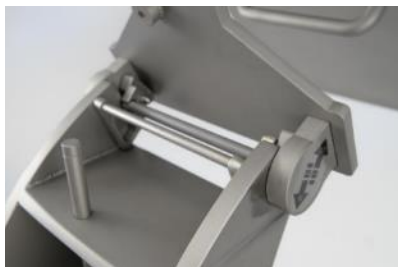
Fig. 21: Fastening the funnel
