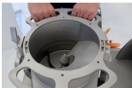
Fig. 28: Inserted screw blade
