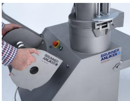
Fig. 43: Attaching the cutting disc holder to the holders on the machine.
