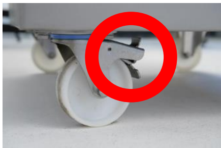
Fig. 12 Parking brake locked in place
