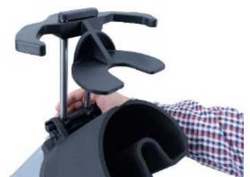
Fig. 37: Snap the plunger in place
