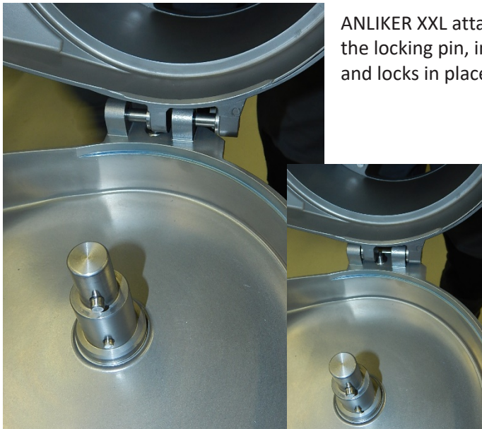
Fig. 13: Mounting the attachment piece
