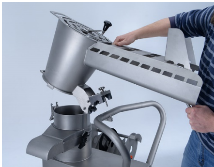
Fig. 15: Mounting the funnel
