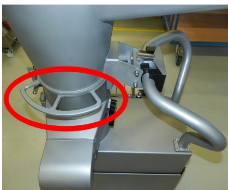
Fig. 26: Moving the screw blades
