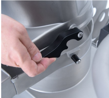
Fig. 14: Locking the attachment piece
