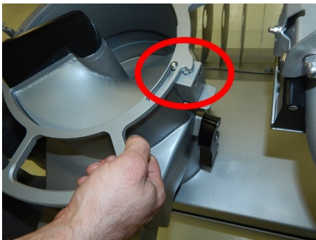
Fig. 22: Inserted screw blade
