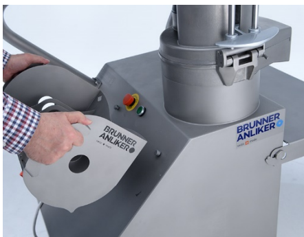
Fig. 30: Hooking up the cutting disc holder on the fastening elements on the machine.
